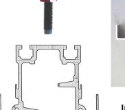
Type 35\* Hufcor Aluminum Track 4-7/8" exposed surface \*(3 degree riding surface angle
