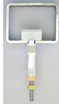
Step 3: Secure a. Release bolt so that head comes downward to seat on riding surface of the track b. Tighten barrel nut to lock TITAN in position
